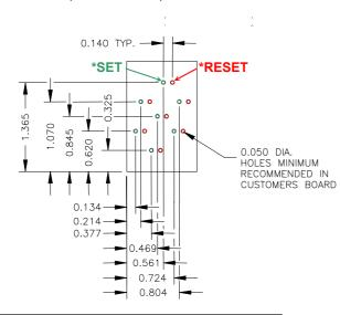
**+SET to -RESET** current direction through the coil will cause the segment to be displayed. **+RESET to -SET** current in the opposite direction through the coil will cause the segment to be hidden.
